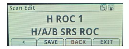
While in Scan Edit mode, pressing the channels currently assigned to the scan list. Once the desired channel is selected press the < key and then Save. The (S) in the upper right display corner designates the channel has been added to the scan list.
